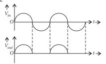
During negative half cycle of input a.c., end A of the secondary winding becomes negative and end B positive. Thus, diode D becomes reverse biased and does not conduct any current. So, no current flows in the circuit. Since electric current through load  $R_I$  flows only during positive half cycle, in one direction only *i.e.*, from A to B, so d.c. is obtained across  $R_I$ .
