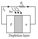
When an external load  $R_L$  is connected as shown in figure, a photocurrent  $I_I$  begins to flow through the load.
