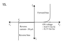
The reverse current is due to minority charge carriers and even a small voltage is sufficient to sweep the minority carriers from one side of the junction to the other side of the junction. Here the current is not limited by the magnitude of the applied voltage but is limited due to the concentration of the minority carrier on either side of the junction.
