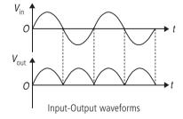
Since in both the half cycles of input a.c., electric current through load  $R_L$  flows in the same direction, so d.c. is obtained across  $R_L$ . Although direction of electric current
