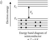
At absolute zero temperature (0 K), conduction band of semiconductor is completely empty, *i.e.*,  $\sigma = 0$ . Hence the semiconductor behaves as an insulator. At room temperature, some valence electrons acquire enough thermal energy and jump to the conduction band where they are free to conduct electricity. Thus the semiconductor acquires a small conductivity at room temperature.
