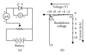
In reverse biased, the applied voltage supports the flow of minority charge carriers across the junction. So, a very small current flows across the junction due to minority charge
